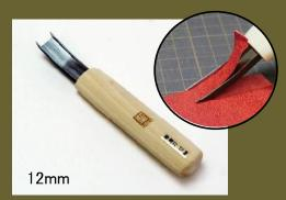
The horn-shaped parts at both ends of the blade double as a guide and guard. You can skive the edges of the leather with the same width.
