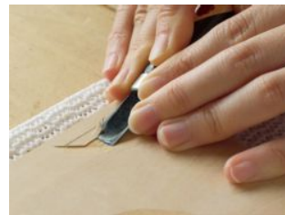
⑦ Tilt the blade and carve along the cut line E and F, as 3. Remove the remained triangle area.
