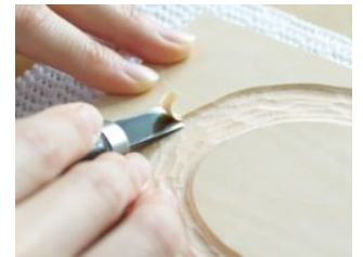
⑧ How to chamfer: tilt the knife (Flat?? 12) and engrave the edge as arrows show in picture 7.
