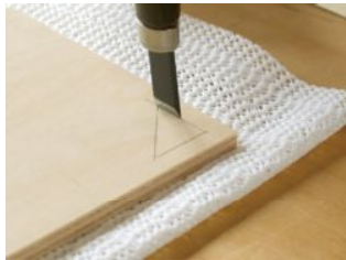
① Set the blade vertically and cut the line A and B.
