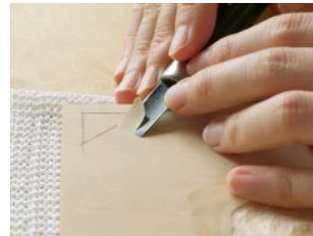
③ As chamfering, tilt the blade and carve along the cut line C.
